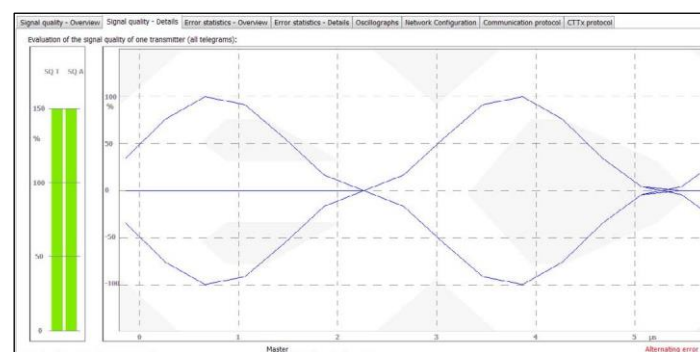
Evaluation of the signal quality for one device „eye pattern“
