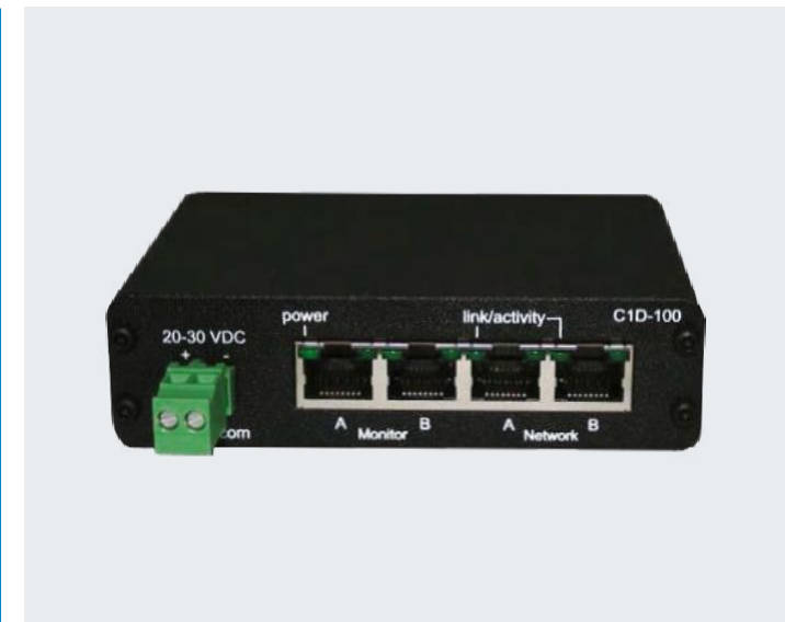
Active measuring point ETMA
