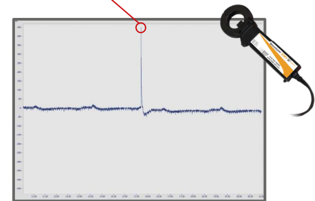
High-frequency glitch at the central supply 24 VDC
